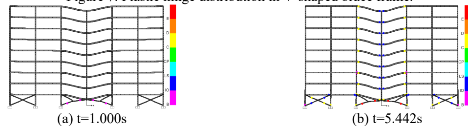
Figure 8. Plastic hinge distribution in X-shaped brace frame.
