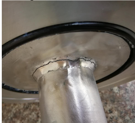
Fig. 2 the crack on the conductive rod of B phase
