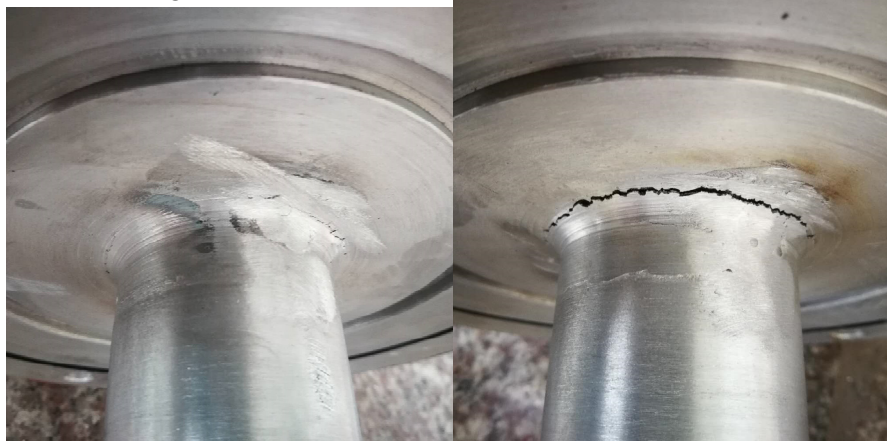
Fig. 3 the crack on the conductive rod of C phase
