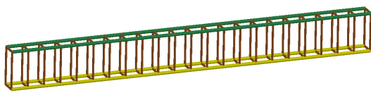
Figure 1. Finite element model of rebar.
