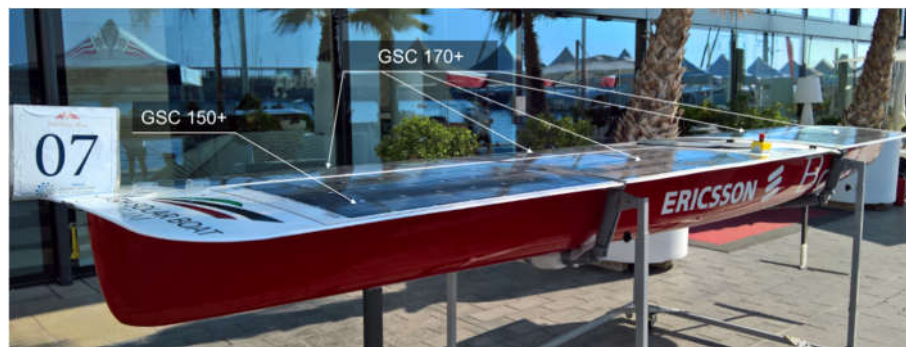
Figure 2. The view of the deck with installed PV panels.
