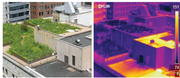
Figure 1. Temperature difference between green roof and traditional roof - Chicago City Hall [11].
