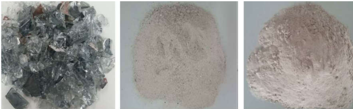
Figure 1. Crushed CRT cullet a) initially crushed, b) milled, c) milled and crushed twice in disintegrator.
