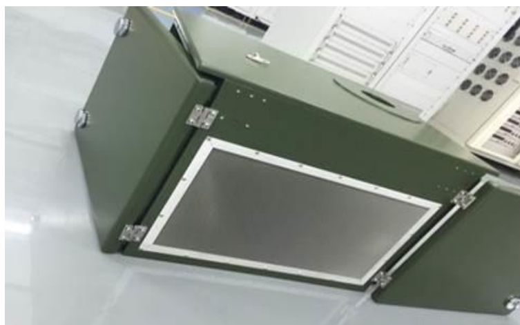
Figure 4. Cut-off waveguide vent used in the chassis air vent.
