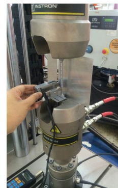
Figure 6: Method of observing magnetic signal offline using aluminium platforms
