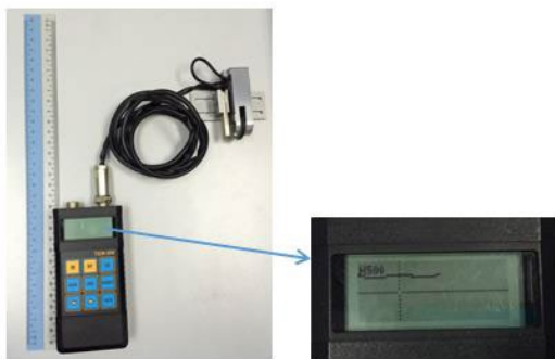
Figure 5: Stress concentration test device and display of the stress concentration graph on screen
