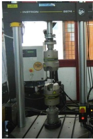
Figure 4: The servo-hydraulic machine used in the study
