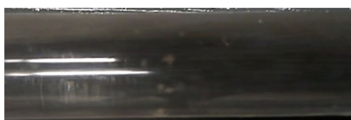
Figure 4(a): The flow inside the pipe without DRA.
