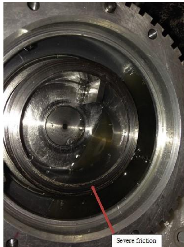
Figure 8. Scratch mark on end face sleeve
