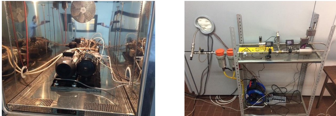
Figure 1. Left: the tested sliding-vane air compressor position inside the climatic chamber. Right: rig to measure and control the delivery pressure as well as to measure the mass flow rate.
