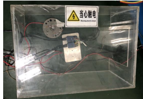
Figure 8 Slip ring calibration bridge circuits
