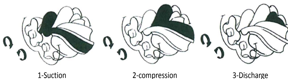
Figure 1 Operating stages in a twin-screw compressor[1].
