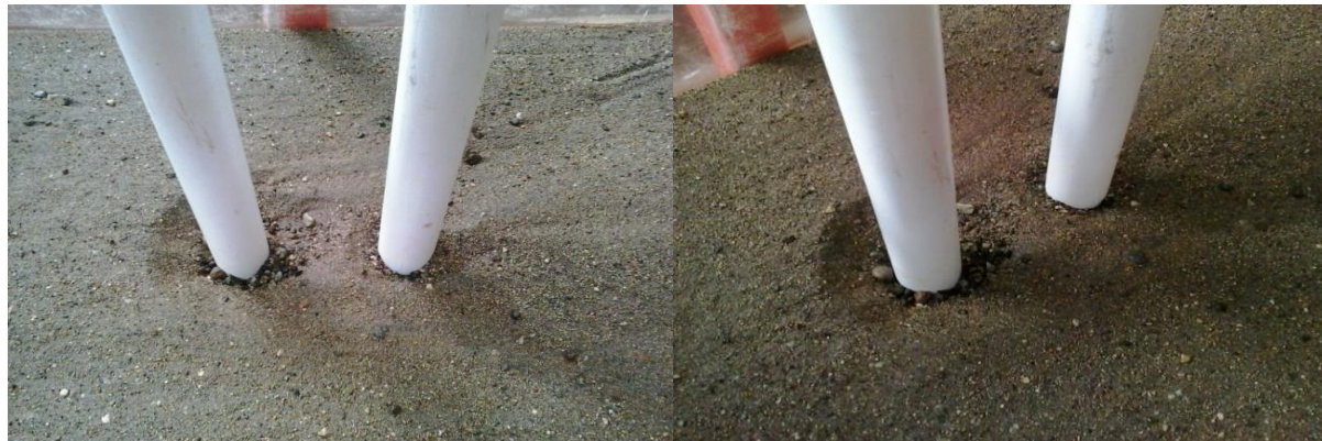
Figure 18. Holes due to scour, and armouring layers around the piers in the position W_1 (left figure) and in the position W_2 (right figure)
