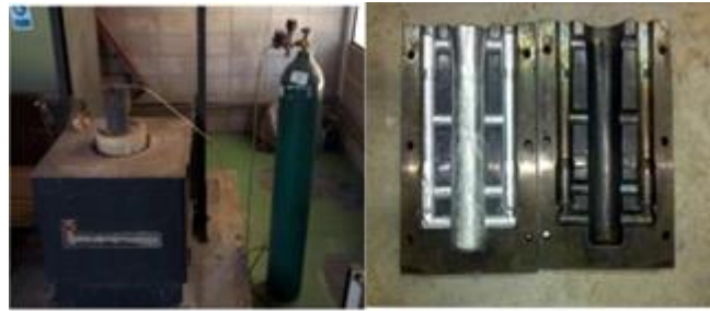
Figure 2. Induction furnace and steel mold
