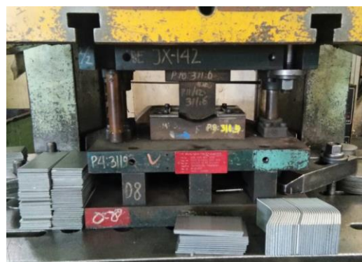
Figure 2. Conventional die construction
