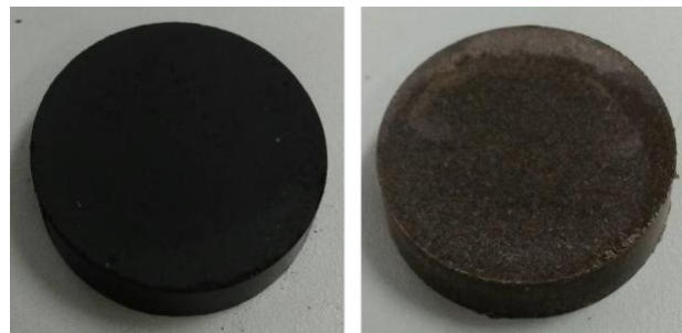
Figure 5. Pallet sample of POFA (left) and BSP (right).
