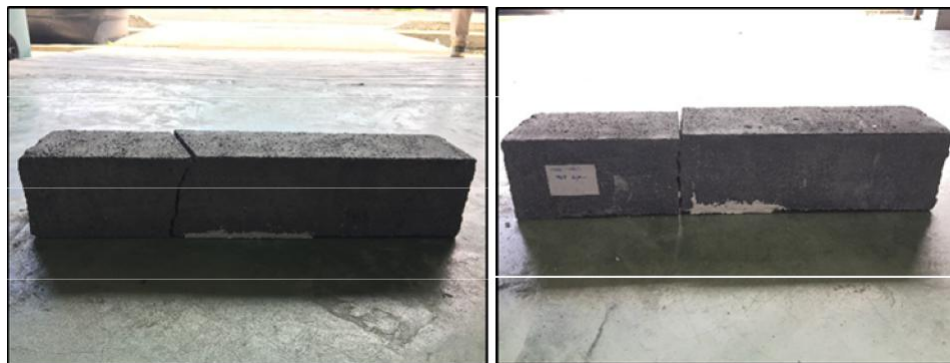
Figure 12. Crack pattern for LFC-BSP-POFA prisms with (a) 100 mm, and (b) 150 mm CFRP.
