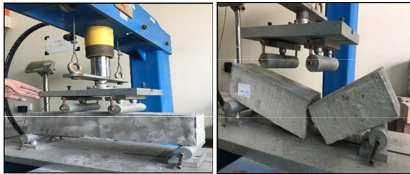
Figure 11. Four point bending load test on prism strengthened with CFRP.
