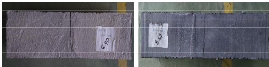
Figure 10. Crack pattern of LFC-BSP-POFA without CFRP strengthening with (a) (0% BSP 15% POFA), and (b) (1% BSP 15% POFA).
