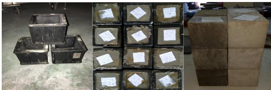
Figure 3. Cubes mould (left), wet mix LFC-BSP-POFA in the mould (center), the LFC-BSP-POFA once demoulded (right).
