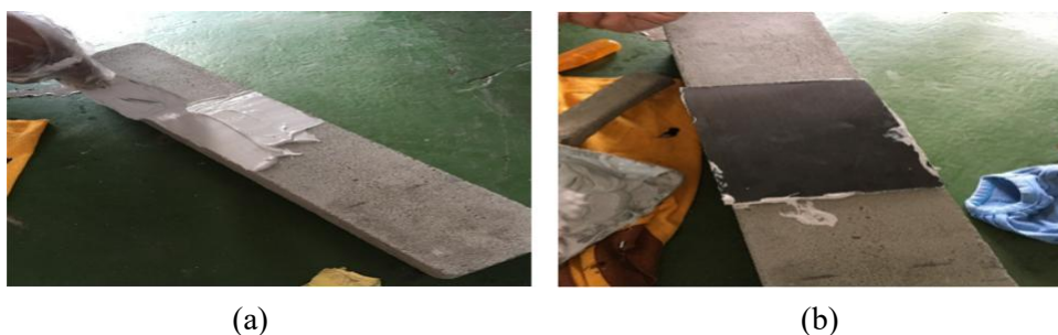
Figure 4. (a) Epoxy paste spread onto the prism surface (b) CFRP glued onto the paste at the bottom surface of the prism.
