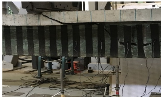
Figure 5. Double layers beam after failure.
