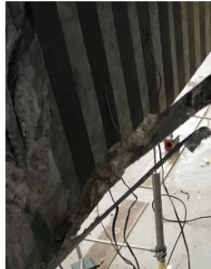
Figure 4. Single layer beam after failure.
