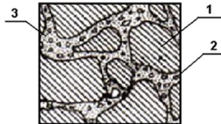
Figure 1. Nanostructurization of cement stone: 1 - cement particles; 2 - ultradispersed quartz waste; 3-hydration products of clinker components.
