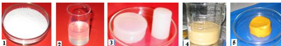
Figure 1. Stages of preparation of filled cryogels: 1 – dry powder of polyvinyl alcohol, 2 – aqueous solution of polyvinyl alcohol, 3 – two-component cryogel, 4 – ‘mineral oil in an aqueous solution of polyvinyl alcohol’ emulsion, 5 – elastic cryogel containing water, polyvinyl alcohol, and mineral oil.
