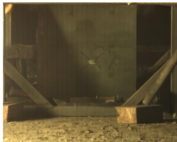
Figure 3. Figure of cracking after explosion with primary source of lighting (aluminium powder).
