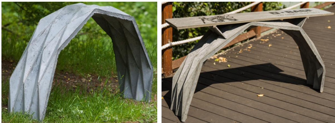
Figure 12. FRC origami bridge.
