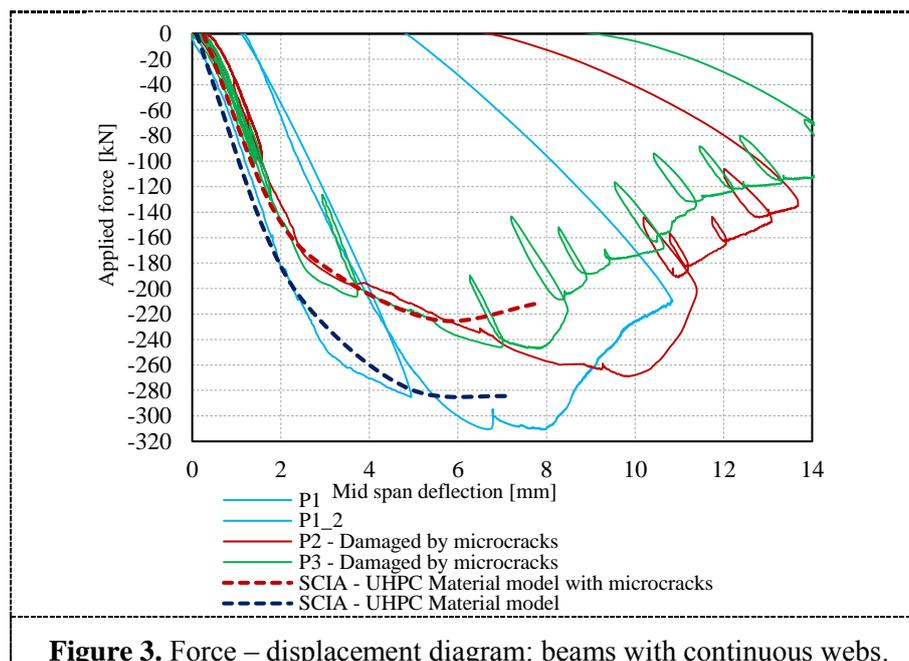
**Figure 3.** Force – displacement diagram: beams with continuous webs.
