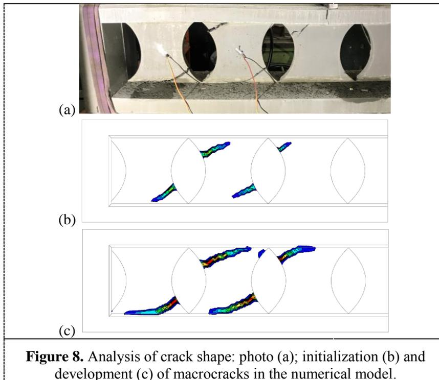
4.3. Comparison of solid and lightened web beams
