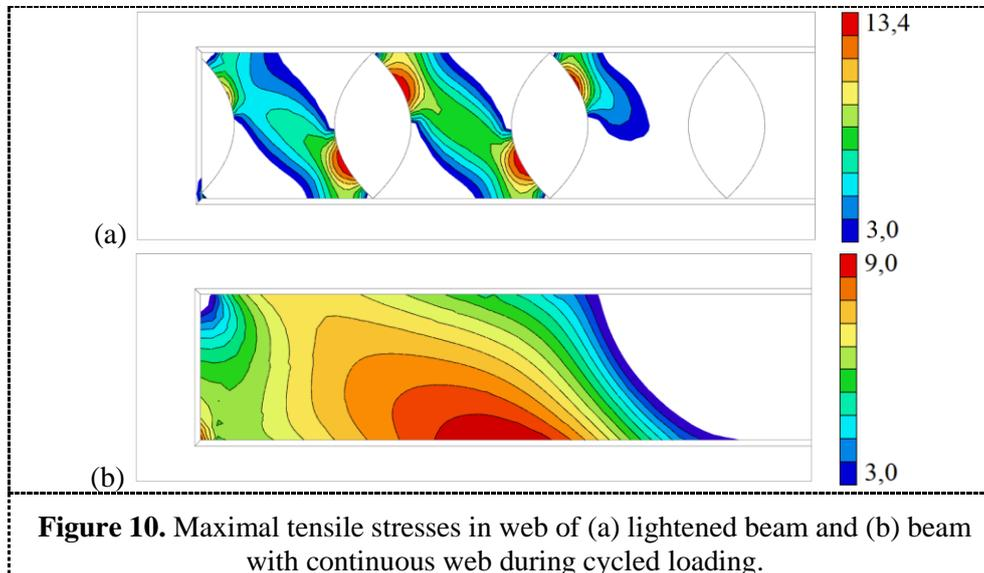
**Figure 10.** Maximal tensile stresses in web of (a) lightened beam and (b) beam with continuous web during cyclic loading.
