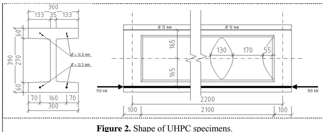
**Figure 2.** Shape of UHPC specimens.
