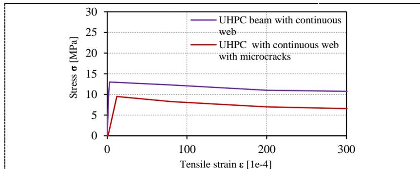
**Figure 4.** Stress – strain diagrams of UHPC – tension.
