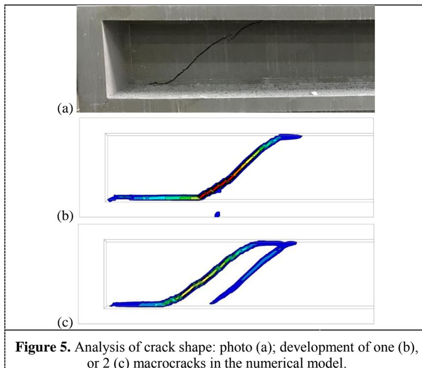
**Figure 5.** Analysis of crack shape: photo (a); development of one (b), or 2 (c) macrocracks in the numerical model.
