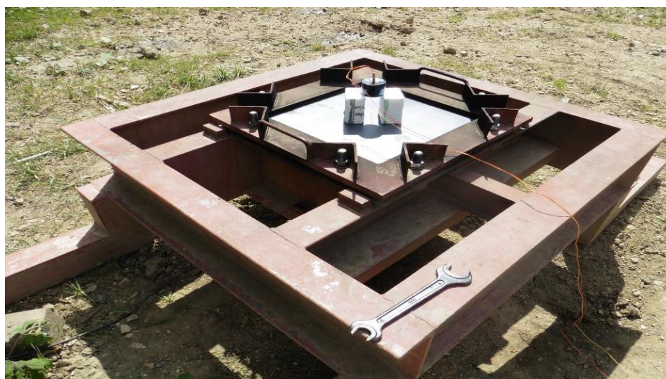
Figure 1. Testing bench T0B and test configuration according to modified method M-T0 VTUO 10/09.
