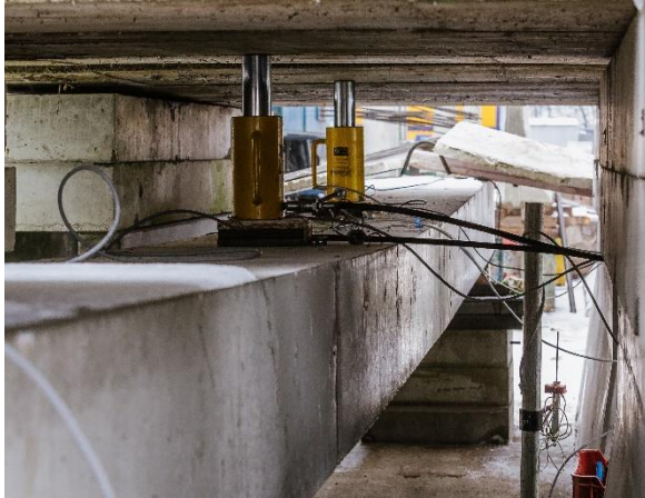
Figure 8. Deflected beam during load test
