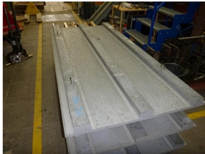
Figure 12. Ribbed deck of lost formwork
