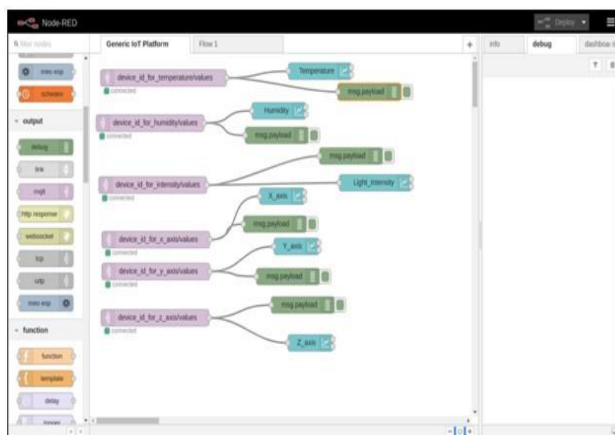
Fig.5 Flow in node red for changing sensor values
