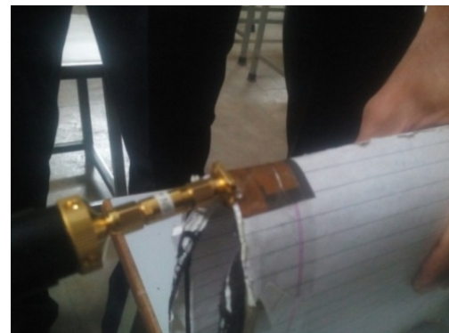
Figure 22 Measurement setup for conformal UWB antenna (bending radius- 25 mm)
