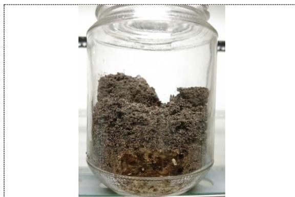
**Figure 1.** Subterranean termite test specimen.
