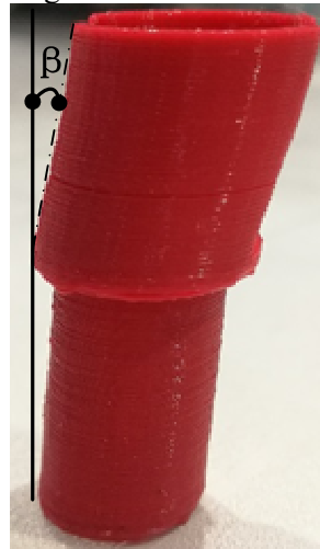
Figure 3. Vibration causes misalignment &amp; skew
