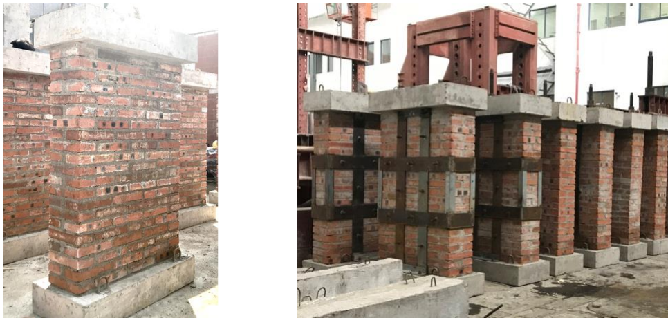
Figure 3. Partially fabricated test specimens
