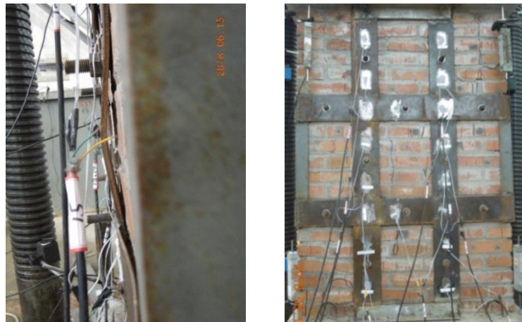
(a) local buckling of steel strips (b) Cracks in the masonry wall
