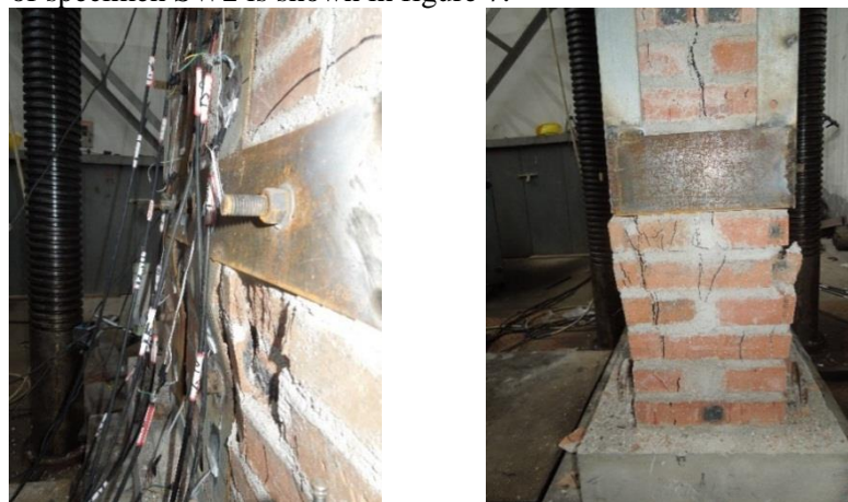
(a) local buckling of steel strips (b) crushing of masonry
