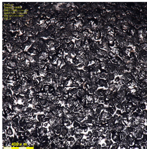
Figure 6 The beryllium sample surface after rough machining
