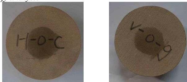
(a) Horizontal bedding (b) Vertical bedding Figure 5. Apparent characteristics of rock at normal temperature
