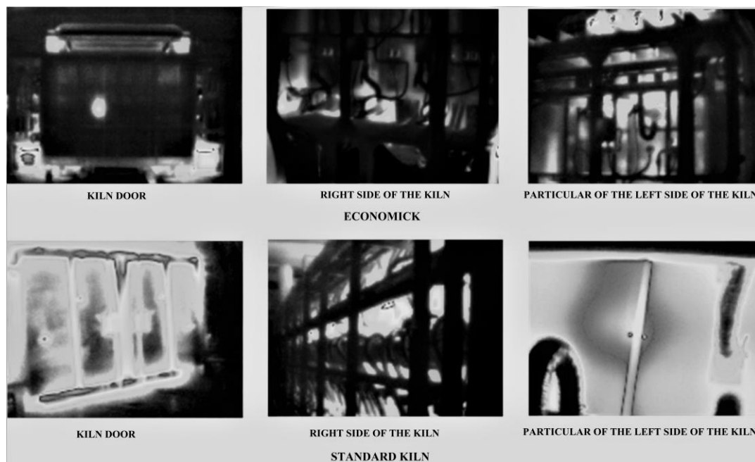
Figure 2. Thermograms obtained in ECONOMICK and standard kiln.
