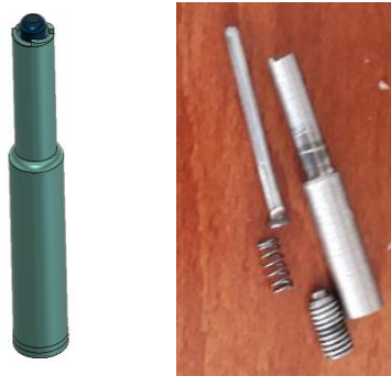
Figure 8. The final tool with a condenser cutter on the tool head.
