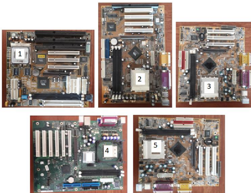
Figure 6. Standard ATX motherboards with liquid dielectric electrolytic capacitors.
