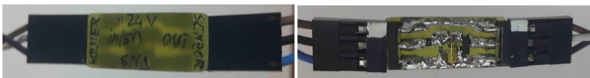
Figure 4. Implementation of the electrical circuit for inductive proximity sensor activation.
