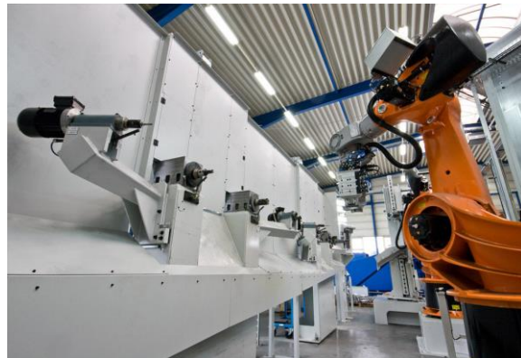
Figure 2. The part being manipulated by the robot and the tool being placed on a work post in a machining application.
