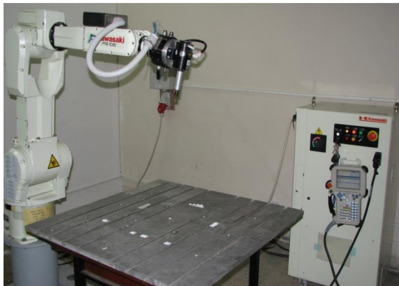
Figure 3. Kawasaki FS10E articulated-arm robot and Kawasaki D controller.
