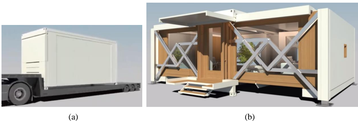
Figure 3. Mobile house in: (a) compact configuration (on a trailer); (b) deployed configuration [9].
