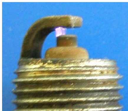
Figure 1. Photo of the spark plug and of the spark discharge.
