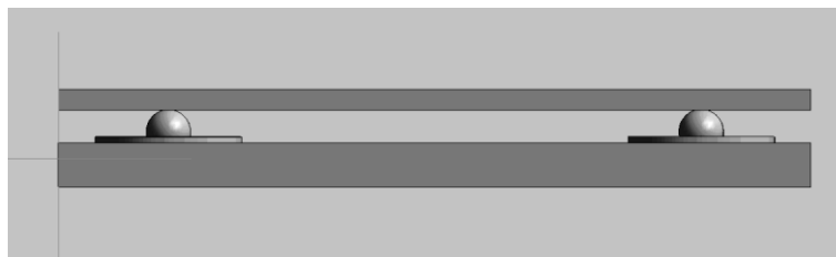
Figure 2. Experimental stand model with rolling isolation system mounted.
