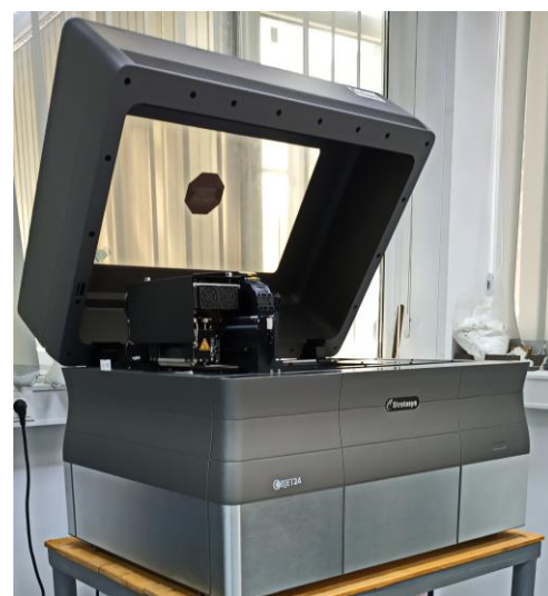
Figure 5. ObJet 24 3D printer produced by Stratasys.
