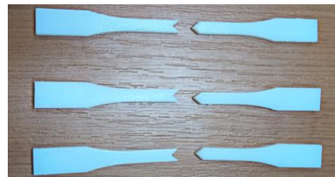
Figure 3. Test specimens for joining tests (VeroWhitePlus FullCure 835).
