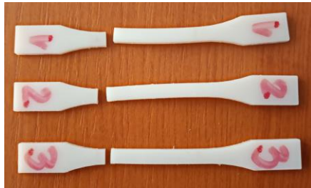
Figure 6. Test specimens of the VeroWhitePlus FullCure 835 material after being required for traction.
