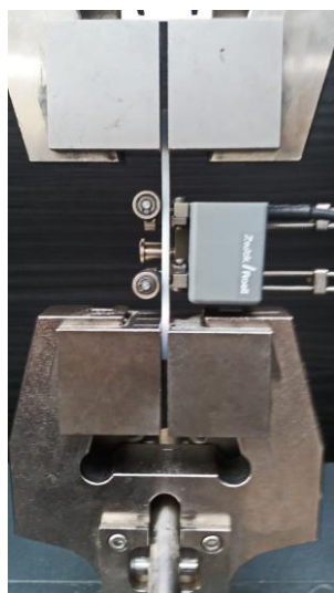
Figure 4. Universal testing machine, load cell of 5kN, Zwick / Roell Z005.
