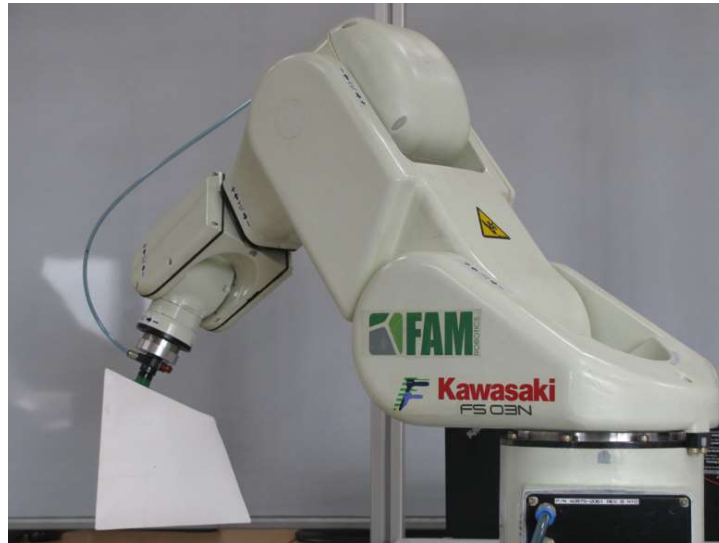
Fig. 1. Kawasaki FS03N robot with the workpiece mockup in the initial pose a
