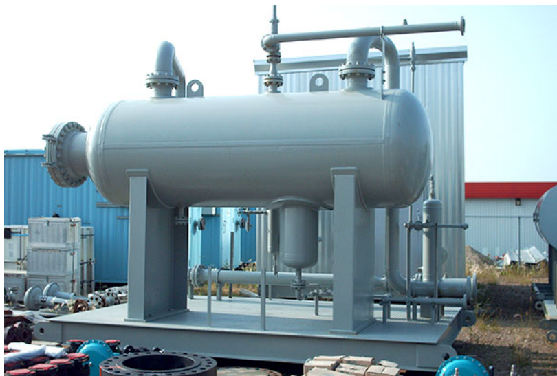
Fig. 1. Example of a gas separation plant
