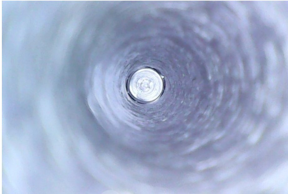
Figure 12. The path of heat exchanger made from AMg6 [93,5% Al, 5,5% Mg], operating time is 100 hours, there are no corrosion signs (there are signs of treatment)
