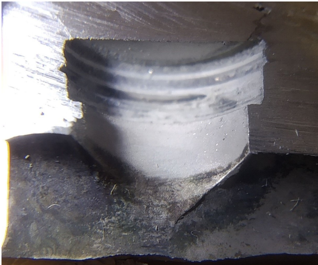
Figure 11. Corrosion zones in the path with and without spray coating
