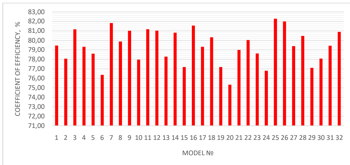
Fig. 3. Pump efficiency distribution bar chart depending on the number of design model for z=9 .
