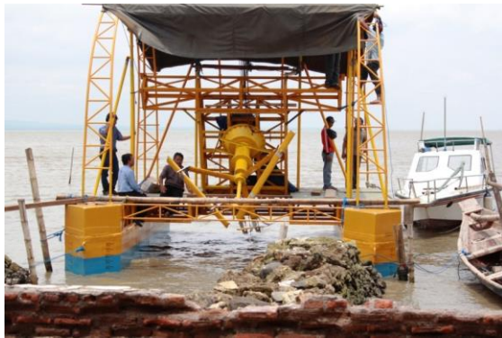
Figure 8. Prototype of wave current rotor
