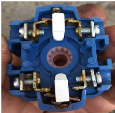
Figure 1. Defects of CA10 series far and near control switches
