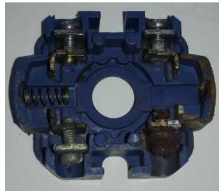
Figure 1. Defects of CA10 series far and near control switches
