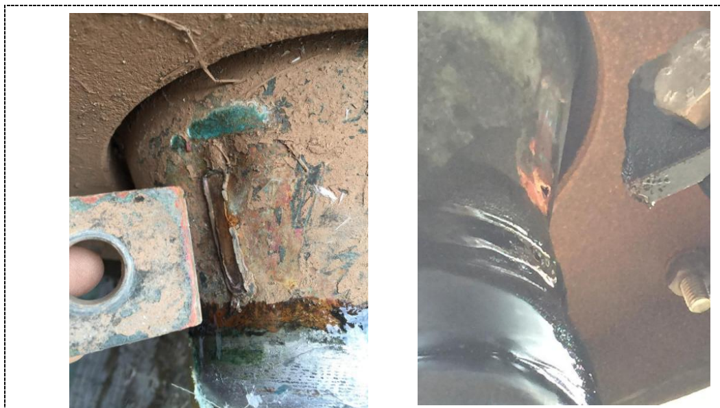
Figure 1. (a) Ground copper block and tail pipe copper are completely separated; (b) Cable terminal tail pipe copper weld zone is cracked.
