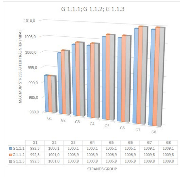
Figure 23. Maximum tension stress in the strands after transfer for beams G 1.1.1, G 1.1.2, G 1.1.3
