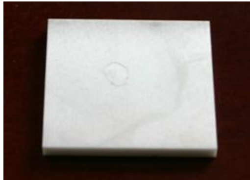
Figure 5. Annular fracture formed by weakened reflected wave (42J)
