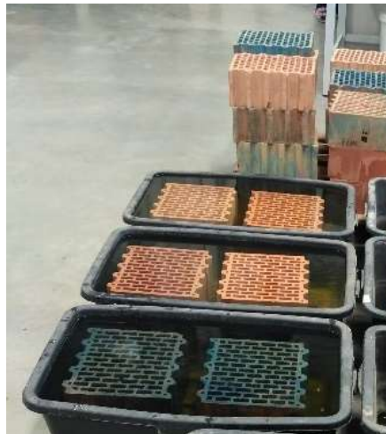
Figure 2. Placing of blocks in a water bath - determination of capillary absorption.
