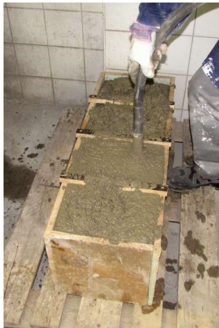
Figure 1. Manufacturing of a prism of 300 \times 300 \times 900 mm (P300).
