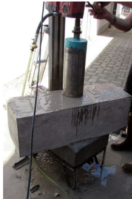
Figure 2. Drilling cores from prism P300.
